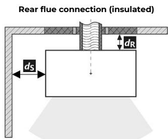
**Passage of the flue pipe through a wall made of combustible material**
